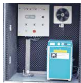
Cabinet with screw compressor and an integrated pump control
